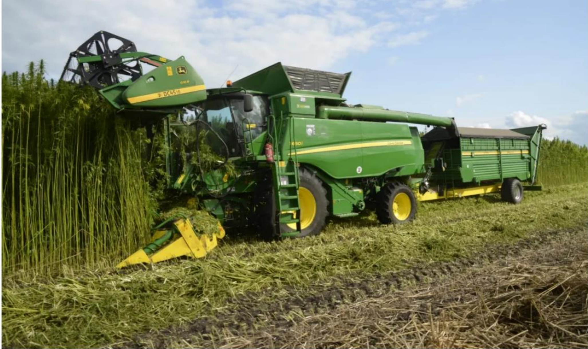
Dutch John Deere dealer Groenoord has developed a trailer to collect hemp leaves harvested by the modified John Deere Double Cut combine.
